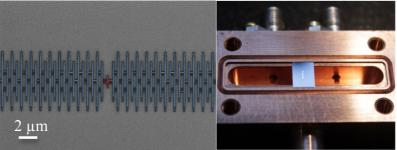
Left: example of a Josephson meta-material we engineer in our lab. It is made of thousands of Josephson junctions and behaves as a "superinductance", which is several orders of magnitude larger than what is usually found in standard electronic circuits. Right: superconducting qubit embedding a superinductance (black rectangle) sitting in its copper microwave cavity. In this specific case, the addition of a superinductance enabled a novel readout mechanism.
